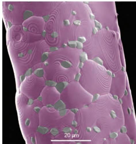
Athina Markaki and T.W. Clyne, 'Surface Steps on a Stainless Steel Fibre'
