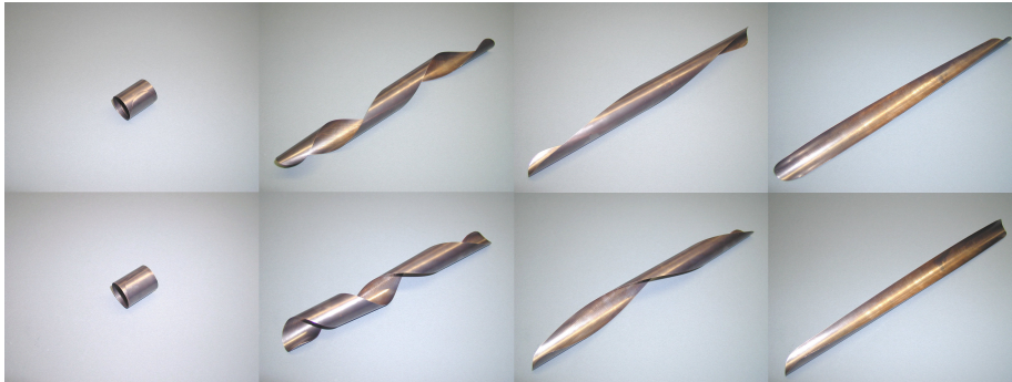
Figure 4: A neutrally stable cylindrical shell [25] can be twisted from fully coiled to fully extended configuration and again to fully coiled (clockwise from top-left) with zero stiffness. In all deformed configurations the shell can be wrapped around an underlying cylinder with constant radius.
