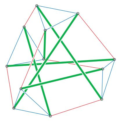
*Figure 3. Tensegrity structure with T symmetry. The outer net of members shown by thin lines (blue and yellow) are cables in tension and the inner bars shown by thick lines (green) are struts in compression.*
