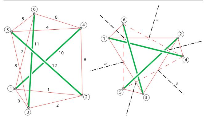
**Figure 1.** Example tensegrity structure with  $D_3$  symmetry. (a) Isometric view, showing the node and element numbering scheme used. Tension members are shown by thin lines, compression members by thick lines. (b) Plan view, showing the top triangle by dashed lines, bottom triangle by solid lines, and the location of three  $C_2$  rotation axes, a, b, c, each of which lies at half height in the structure.
