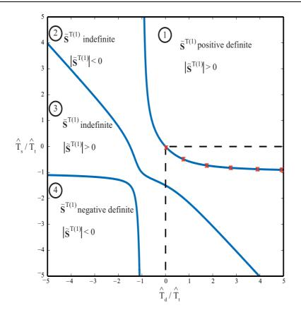
**Figure 4.** Solutions of Eq. 17,  $|\widetilde{\mathbf{S}}^{\mathbf{T}_1}| = 0$ . The solutions lie on three lines, which split the plot into 4 regions. Requiring  $\mathbf{S}$ , and hence  $\widetilde{\mathbf{S}}^{\mathbf{T}_1}$  to be positive semi-definite implies that we are interested in the solution between regions (1) and (2). Additionally requiring  $\hat{T}_d / \hat{T}_t$  positive, and  $\hat{T}_s / \hat{T}_t$  negative, gives solutions marked by crosses.
