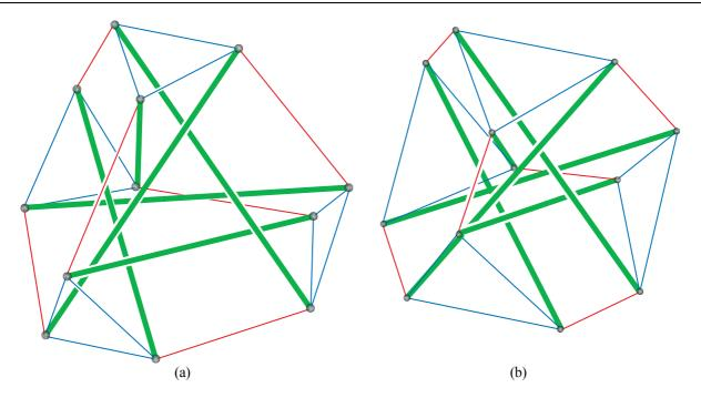
Figure 5. Possible configurations of Tensegrity structures with T symmetry.
