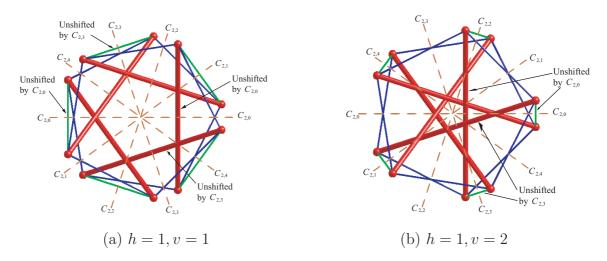
Fig. 2. Structures  $\mathbf{D}_n^{h,v}$  with n(=5) odd. One strut and one vertical cable remain unshifted by any two-fold rotations, and all are shifted by any *n*-fold rotations except the identity operation.
