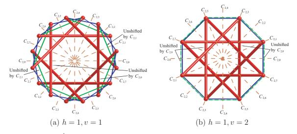
Fig. 3. Structures  $\mathbf{D}_{n}^{h,v}$  with n(=8) even. Two struts remain unshifted by a two-fold rotation  $C_{2,2i}$ , and all struts are shifted by  $C_{2,2i+1}$ . For v odd, all vertical cables are shifted by  $C_{2,2i}$ , and two are unchanged by  $C_{2,2i+1}$ . For v even, two vertical cables are unshifted by  $C_{2,2i}$ , and all are shifted by  $C_{2,2i+1}$ .
