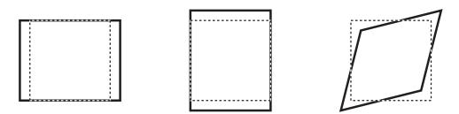
Figure 1: The deformations of the unit cell that are compatible with periodic mobility in 2D, comprising (left to right) two orthogonal stretches and one shear.
