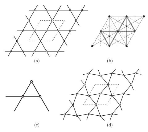
Figure 2: The kagome framework, showing (a) the choice of unit cell used here; (b) the unit cell with symmetry elements denoted by the standard symbols of a rhombus for a  $C_2$  axis, triangle for a  $C_3$  axis, hexagon for a  $C_6$ axis, solid line for a reflection line, and a dashed line for a glide line; (c) a motif with a minimal set of complete joints and bars; (d) a deformed configuration, illustrating the  $B_2$ -symmetric mechanism detected by the analysis reported in Section 4.1.
