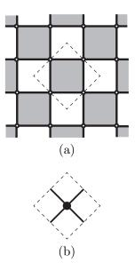
Figure 5: Model for an auxetic material based on squares of equal size, showing (a) the model and the smallest choice of unit cell with rigid plates indicated by shading; (b) the contact polyhedron C for the unit cell which in this case consists of a single unique vertex.
