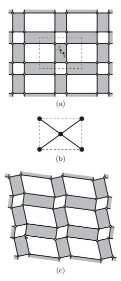
Figure 4: Model for an auxetic material based on rectangles of two sizes, showing (a) the model and the choice of unit cell with rigid plates indicated by shading; (b) the contact polyhedron C for the unit cell; (c) a deformed configuration, illustrating the  $A_2$ -symmetric mechanism.
