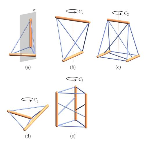
Figure 5: Isostatic symmetric rod-bar frameworks, with their point-group symmetries ((a)  $\mathcal{C}_s$ ; (b),(c),(d)  $\mathcal{C}_2$ ; (e)  $\mathcal{C}_3$ ), exemplifying the various structural counting rules derived in the text.
