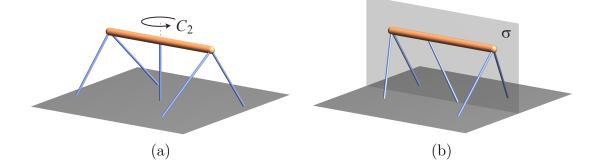
Figure 8: Two symmetric configurations of the linear pentapod, one with half-turn symmetry (a) and one with reflection symmetry (b).
