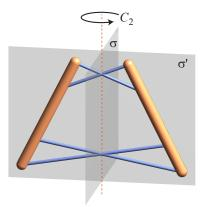
Figure 9: A rod-bar framework with  $C_{2v}$  symmetry. As it lies within the mirror plane corresponding to  $\sigma'$ , it is not isostatic.
