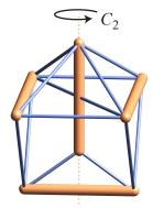
Figure 3: A rod-bar framework with an isostatic scalar count that has an infinitesimal motion and a state of self-stress, both detected by calculations of the symmetry-extended mobility count. In this and subsequent figures, rods are schematically depicted as 'wooden', and bars as 'metallic'.
