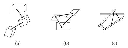
Figure 1: Frameworks in 3-space: (a) A *body-bar* framework, (b) a *panel-bar* framework, and (c) a *rod-bar* framework. Dumbbell symbols indicate a bar and its two points of attachment.
