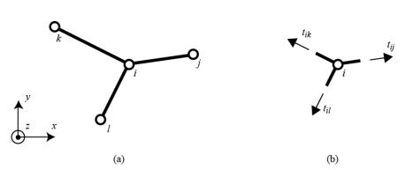
Figure 4: (a) shows four nodes connected by three members; (b) shows a free-body diagram of the central node.
