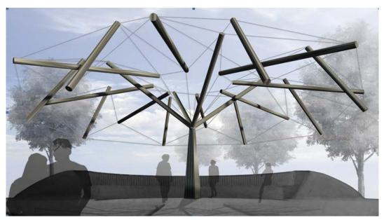
Figure 1: Tensegritree sculpture render. The structure has a height of 7 m, and a diameter of 12 m
