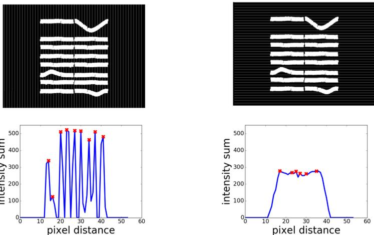
Fig. 1: Perpendicular lines drawn on the binary image at angle 0° (left) and 90° (right), along with their oriented graphs of intensity sums.
