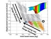
Trailer light-weighting: geometry optimisation of steel chassis beams
