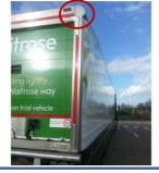
Aerodynamic improvements on in-service test trailer
