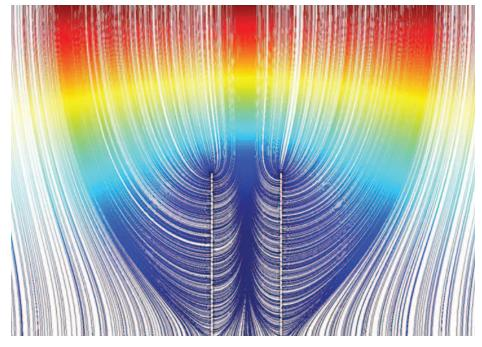
Simulation of the electric field surrounding a single MWCNT in vacuum
