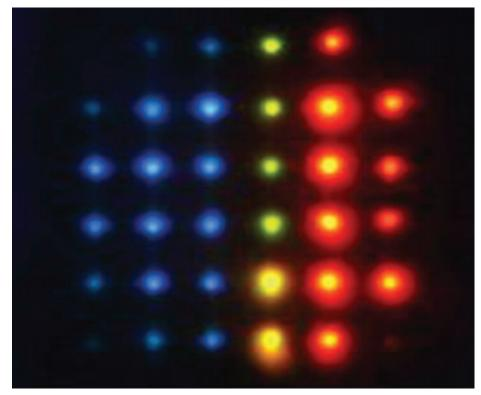
Polychromatic laser emission from a gradient pitch liquid crystal cell, pumped from a single optical source
