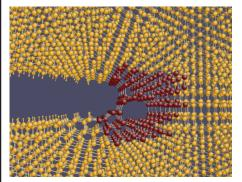
Special configuration of the tip of a crack in silicon
