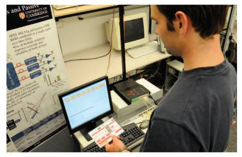
Researcher Michael Crisp demonstrating the TINA passenger location system whereby the passenger is tracked via monitoring of an RFID tag on the boarding card
