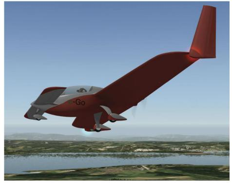
The stabiliser is at the front, which prevents stalling and minimises weight. The two projects optimised the aerodynamic interaction between the canard and the wing.
