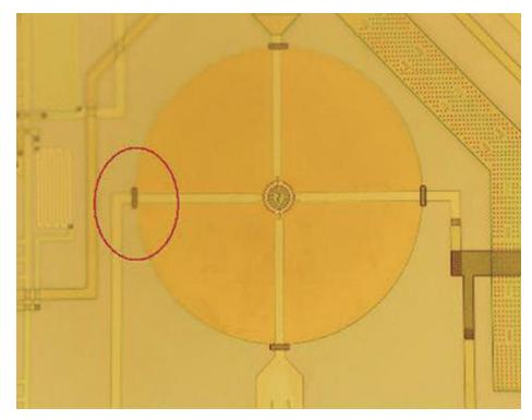
Photograph showing an SOI microhotplate (large circle) with a small micro-heater (12 micron radius) and integrated tempertaure sensor. DC power consumption is a few milliwatts at 300 C and tens of microwatts when operated in a pulsed mode. Red ellipse indicates very accurate back etch with alignment mark.
