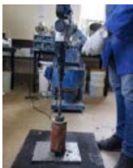
Fig 1. Dynamic vibration hammer for the compaction and moulding of RCC cylindrical specimens
