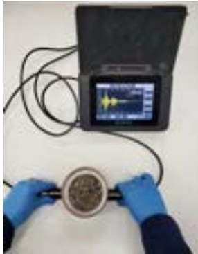
Fig 3. Proceq ultrasonic device to measure the RDME and concrete internal structural damage due to freeze-thaw
